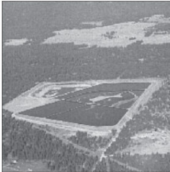
An aerial photo shows over 100 acres of evaporation ponds being used to remove polluted water from the local aquifer.
